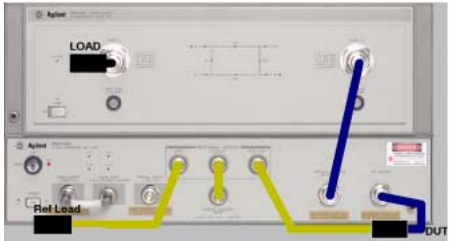
Figure 4-28. Connection for E/O Reflection Sensitivity Calibration (Std1)
