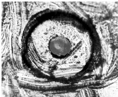
Figure 2-16. Damage from improper cleaning.
