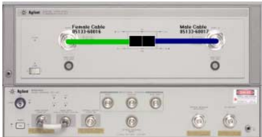
Figure 4-18. Connections for O/E Response and Match Calibration (Std8)
